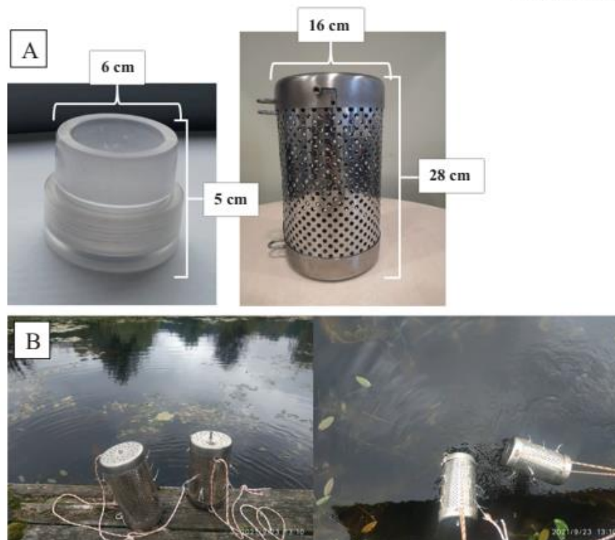
Fig. 3. A - Pictures and dimensions of home-made passive sampler and stainless steel canister. B - Pictures from deployment of passive samplers immersed to a depth of ~2 m in Lake in Sztumskie Pole.
